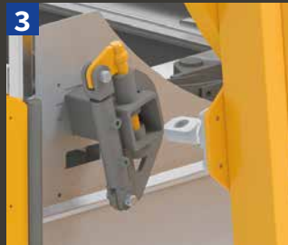
3 Locking mechanism less susceptible to dirt, adjustable and durable
